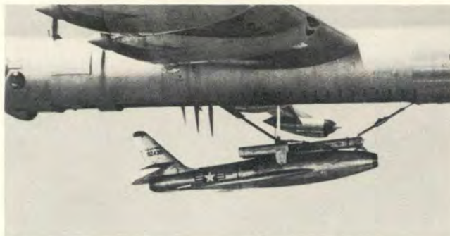
With the aircraft securely anchored to the boom mechanism, operators in the big bomber start hoisting the "84" upward.
