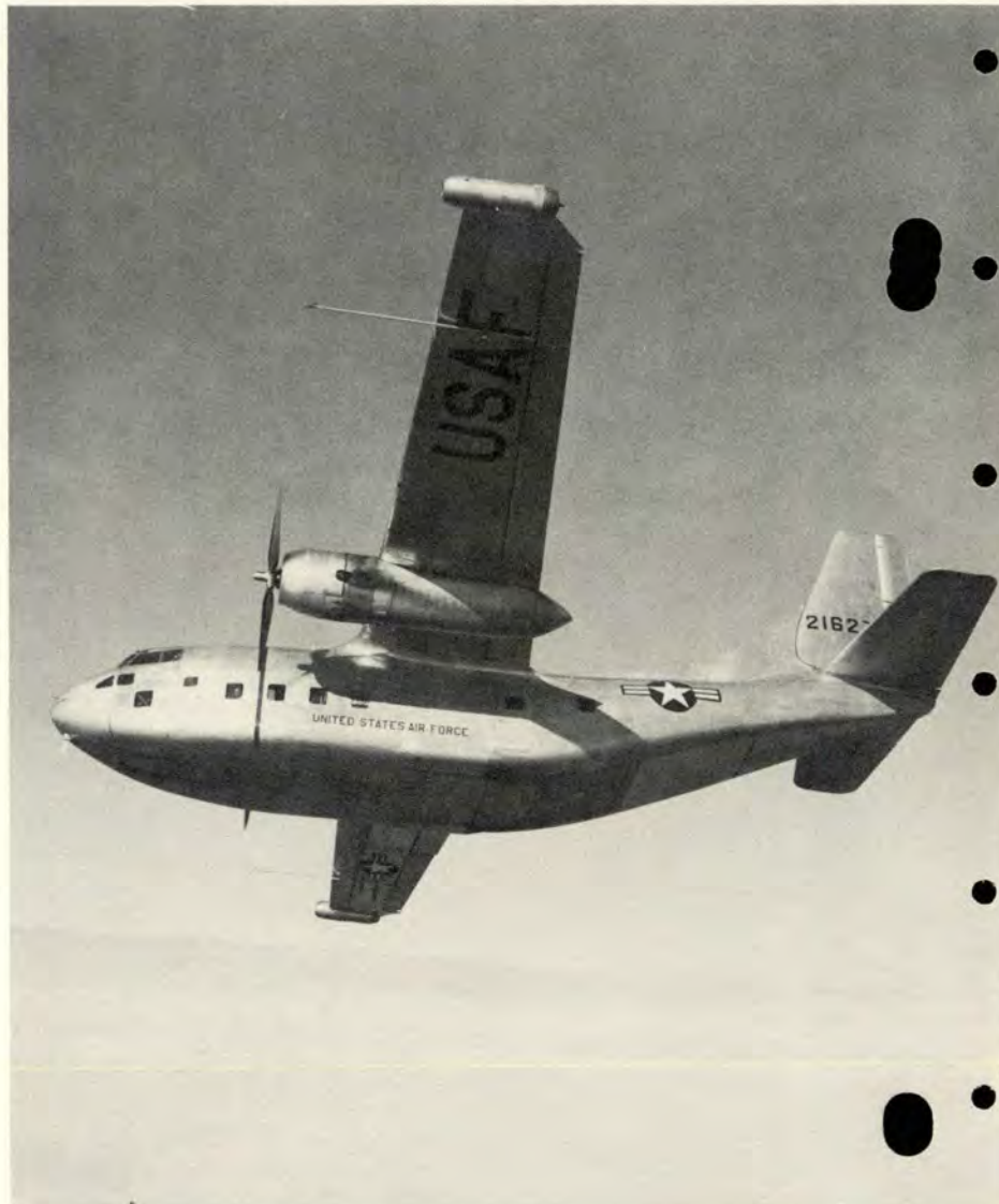
J-44 jets add 2000 pounds of thrust, greatly increasing both takeoff and emergency performance.
