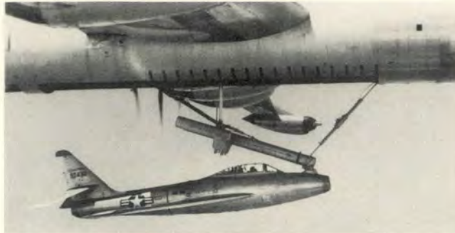
A probe on the nose of an F-84 fighter engages the boom of an RB-36 as initial contact in the mid-air hook-up is made.
