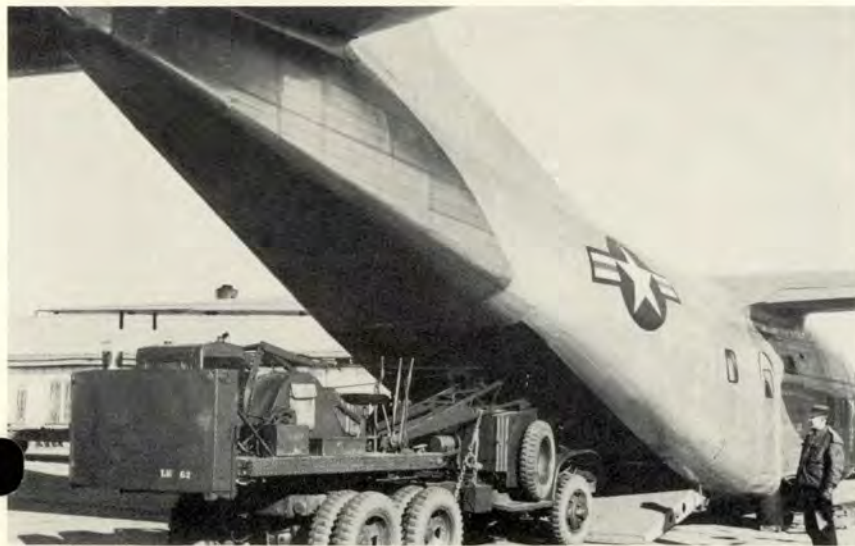
Wheeled vehicles and artillery pieces are loaded or unloaded without cargo handling equipment.
