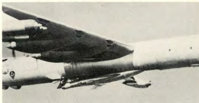
The "landing" completed, the fighter is snuggled into the belly of the "36" where it can remain or be launched again.
