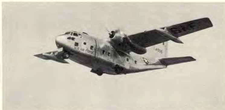
The C-123 has the capability of operating in and out of short, rough fields. Even without the two J-44s, the two Pratt and Whitney R-2800s enable this aircraft to take off quickly fully loaded.
